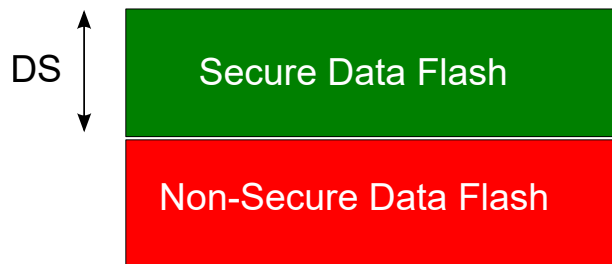
Figure 13-3. SAM L11 Data Flash Memory Mapping
