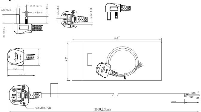
CABLE MARKING: H05VV-F 3G1. 5mm² ◀ VDE ► N19626 CCC A030116 No. 2003010105097406 227 IEC 53 (RVV) 300/500V 3X1. 5mm² H1GH PROJECT LF
