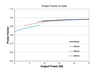
OT FIT 20 CS T Typical Power Factor vs. Load
