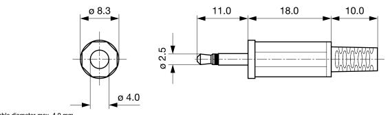
Cable diameter max. 4.0 mm
