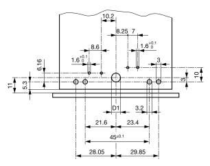
Fixation on PCB or housing from below
