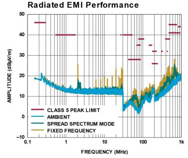
Figure 2. LT8641A Eval Circuit Conducted and Radiated EMI Performance in CISPR25 Emission Test (V<sub>EMI</sub> = 14V, V<sub>OUT</sub> = 5V, I<sub>OUT</sub> = 3.5A, 2MHz Switching Frequency)
