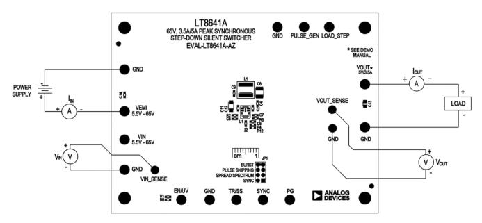
Figure 3. Proper Measurement Equipment Setup
