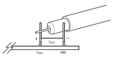
Figure 4. Scope Probe Placement for Measuring Input or Output Voltage Ripple
