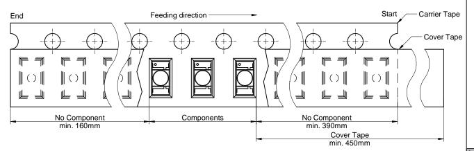
detail B Cover Tape Chip Cavity Sprocket Hole
