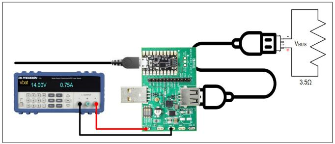
Figure 4. EV Kit Setup for Cable Compensation
