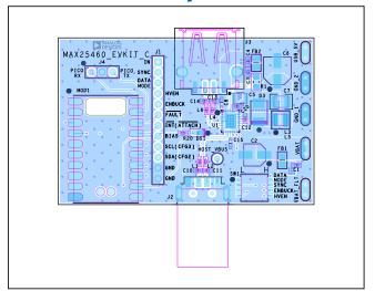
MAX25460 EV Kit PCB Layout—Top View
