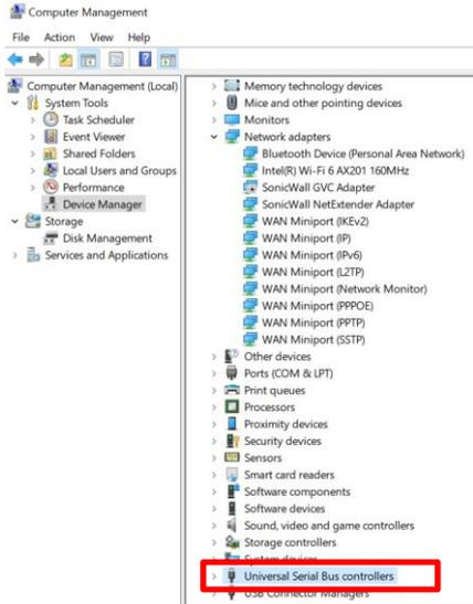
※If you do not see the USB demo board plugged into the "Universal Serial Bus (USB) Controller", it may be recognized as an unknown device in "Other Devices".
