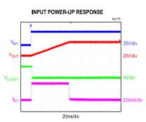
CONDITIONS: V<sub>IN2</sub> = OPEN,  $I_{LIM1}$  = 0.3A,  $C_{OUT}$  = (2\*470µF),  $R_{OUT}$  = OPEN
