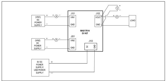
Figure 1. MAX17614 EV Kit Setup Diagram
