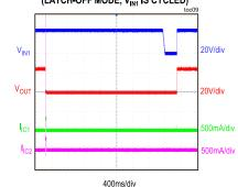
CONDITIONS:  $I_{LIM1}$  =  $I_{LIM2}$  = 0.3A,  $R_{OUT}$  = OPEN TO 1 $\Omega$  (FOR 3s DURATION)
