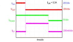
$\begin{array}{c} \text{OUTPUT SHORT-CIRCUIT RESPONSE} \\ \text{t}_{\text{BLANK}} \text{ = } 20\text{ms} \end{array} , \end{array}$
