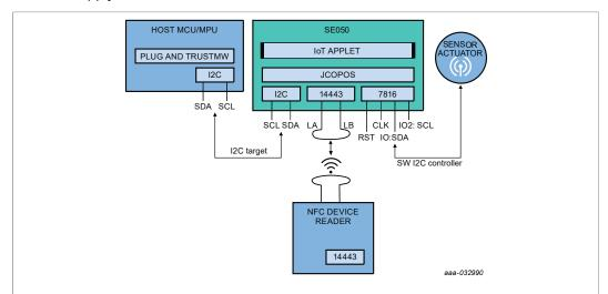
Figure 1. SE050 solution block diagram
