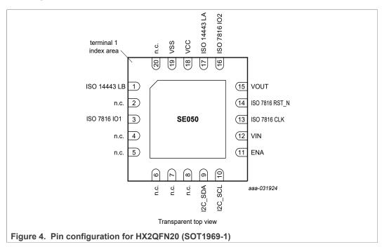
**Note:** Terminal 1 index area is marked on the bottom with a notch on the center pad and on the top with a printed dot.
