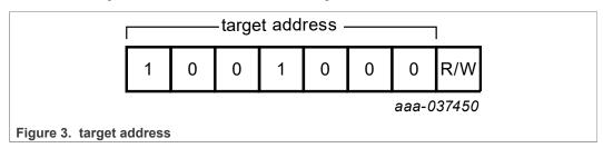
The I<sup>2</sup>C controller interface is supposed to be used with target devices that need to be securely written and read. This interface features a maximum SCL clock rate of 400 kHz.
