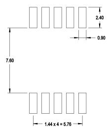
NOTE: All dimensions are in millimeters (mm).
