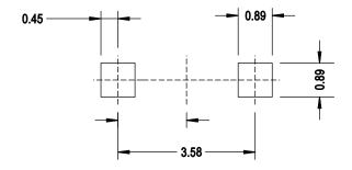
Figure 10: Recommended Soldering Land Pattern for Z-Bend Lead
