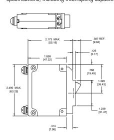
Tolerance ± .015 [.39] unless noted. Dimensions in brackets [] are millimeters. \*See Single Pole Mounting Detail for Hole Sizes and Locations.
