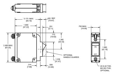
Note: Tolerance  $\pm$  .015 [.38] unless noted. Dimensions in brackets [ ] are millimeters
