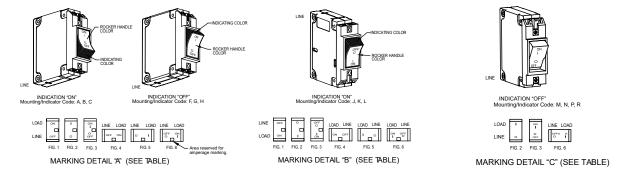
Notes: The LEL family of circuit breakers are designed to meet 8mm creepage and clearance requirements for installation Category 111, pollution degree 3, Case A as measured in IEC 664. Intended for use in equipment designed to comply with IEC 380, 435, 601.
