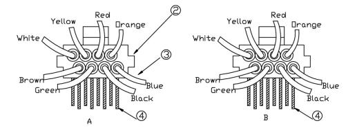
Housing colour: Black Materials: Housing: Polycarbonate Insert: ABS Wire: PVC Contact pin: Gold plated phosphor bronze
