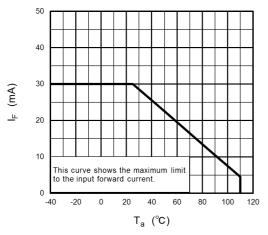
Fig. 12.1.1 I<sub>F</sub> - T<sub>a</sub>
