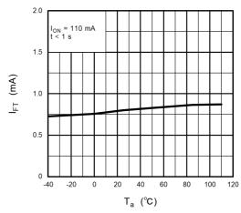
Fig. 12.1.6 I<sub>FT</sub> - T<sub>a</sub>
