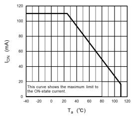
Fig. 12.1.2 I<sub>ON</sub> - T<sub>a</sub>
