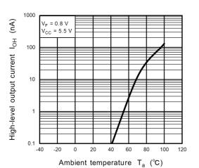
Fig. 13.2.3 I<sub>OH</sub> - T<sub>a</sub>
