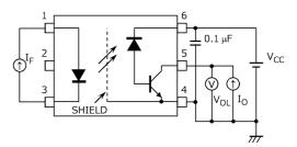
Fig. 13.1.2 V<sub>OL</sub> Test Circuit
