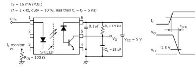
${}^*C_L$  is approximately 15 pF which includes probe and stray wiring capacitance.
