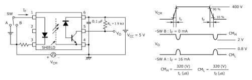
Fig. 13.1.6 Common-Mode Transient Immunity Test Circuit and Waveform
