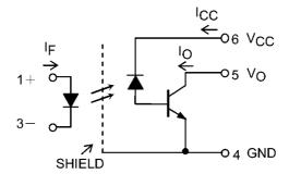
Note: A 0.1- $\mu F$  bypass capacitor must be connected between pin 6 and pin 4.
