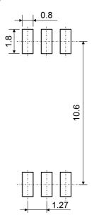
Fig. 15.1 Lead Forming Option (standard)
