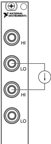
Figure 6. 2-Wire and 4-Wire Resistance
