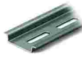
Item no.: 210-504 Steel carrier rail; 35 x 7.5 mm; 1 mm thick; 2 m long; slotted; galvanized; according to EN 60715; silver-colored
