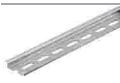
Item no.: 210-115 Steel carrier rail; 35 x 7.5 mm; 1 mm thick; 2 m long; slotted; according to EN 60715; "Hole width 18 mm; silver-colored
