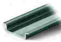
Item no.: 210-113 Steel carrier rail; 35 x 7.5 mm; 1 mm thick; 2 m long; unslotted; according to EN 60715; silver-colored
