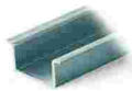
Item no.: 210-506 Steel carrier rail; 35 x 15 mm; 1.5 mm thick; 2 m long; unslotted; galvanized; similar to EN 60715; silver-colored
