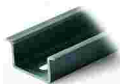
Item no.: 210-508 Steel carrier rail; 35 x 15 mm; 1.5 mm thick; 2 m long; slotted; galvanized; similar to EN 60715; silver-colored
