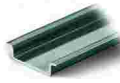
Item no.: 210-505 Steel carrier rail; 35 x 7.5 mm; 1 mm thick; 2 m long; unslotted; galvanized; according to EN 60715; silver-colored
