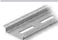
Item no.: 210-112 Steel carrier rail; 35 x 7.5 mm; 1 mm thick; 2 m long; slotted; according to EN 60715; "Hole width 25 mm; silver-colored
