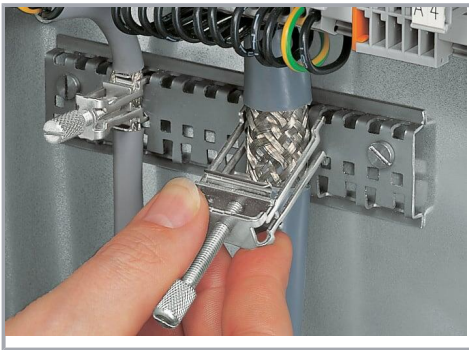
To remove the clamping saddle, unscrew until ratcheted mechanism is released, then slightly tip saddle and remove the clamping saddle.
