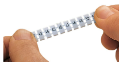
Stretching a WMB marker strip.
