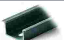
Item no.: 210-508 Steel carrier rail; 35 x 15 mm; 1.5 mm thick; 2 m long; slotted; galvanized; similar to EN 60715; silver-colored
