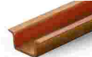
Item no.: 210-198 Copper carrier rail; 35 x 15 mm; 2.3 mm thick; 2 m long; unslotted; according to EN 60715; copper-colored
