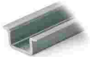
Item no.: 210-118 Steel carrier rail; 35 x 15 mm; 2.3 mm thick; 2 m long; unslotted; according to EN 60715; silver-colored
