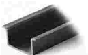
Item no.: 210-114 Steel carrier rail; 35 x 15 mm; 1.5 mm thick; 2 m long; unslotted; similar to EN 60715; silver-colored
