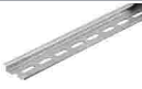
Item no.: 210-115 Steel carrier rail; 35 x 7.5 mm; 1 mm thick; 2 m long; slotted; according to EN 60715; "Hole width 18 mm; silver-colored
