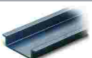
Item no.: 210-196 Aluminum carrier rail; 35 x 8.2 mm; 1.6 mm thick; 2 m long; unslotted; similar to EN 60715; silver-colored
