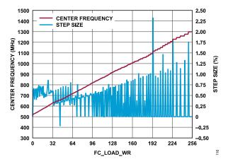
Figure 16. Center Frequency and Step Size vs. FC\_LOAD\_WR
