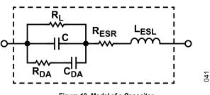
Figure 19. Model of a Capacitor
