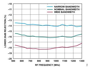
Figure 10. Percentage Away from f<sub>CENTER</sub> for Lower 20 dB Rejection vs. RF Frequency for Various Bandwidths
