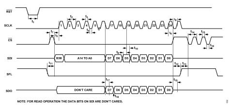
Figure 2. Timing Diagram
