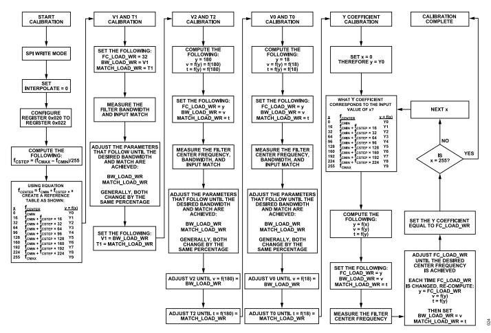
Figure 26. Interpolation Coefficient Calibration Flow Chart
