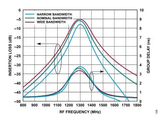
Figure 9. Insertion Loss and Group Delay vs. RF Frequency at 1.3 GHz
