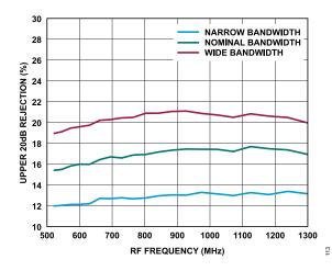
Figure 13. Percentage Away from f<sub>CENTER</sub> for Upper 20 dB Rejection vs. RF Frequency for Various Bandwidths
