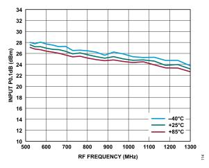
Figure 14. Input P0.1dB vs. RF Frequency for Nominal Bandwidth and Various Temperatures
