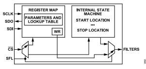
Figure 20. Simplified SPI Diagram
