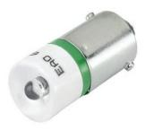
Illuminative colour Operating voltage 130 V AC +10% Operating voltage tolerance +10% % Operation current  $3 \text{ mA} \pm 15 \%$ Operation current tolerance ±15 % % Weight 0.002 kg Illumination colour Green 525 nm Dom. Wavelength Lumi. Intensity 450 mcd
