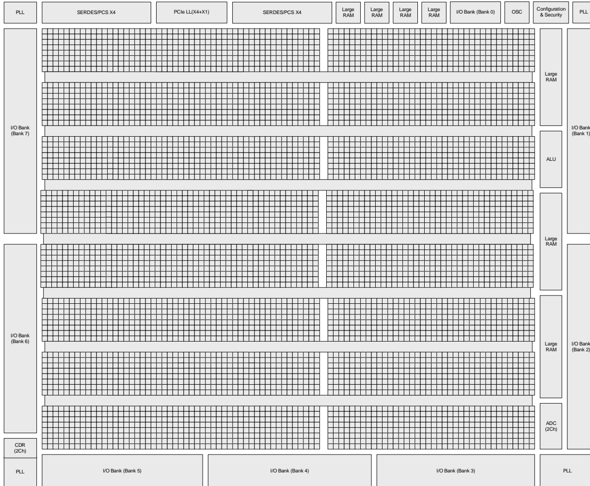
Figure 2.2. Simplified Block Diagram, LFCPNX-100 Device (Top Level)
