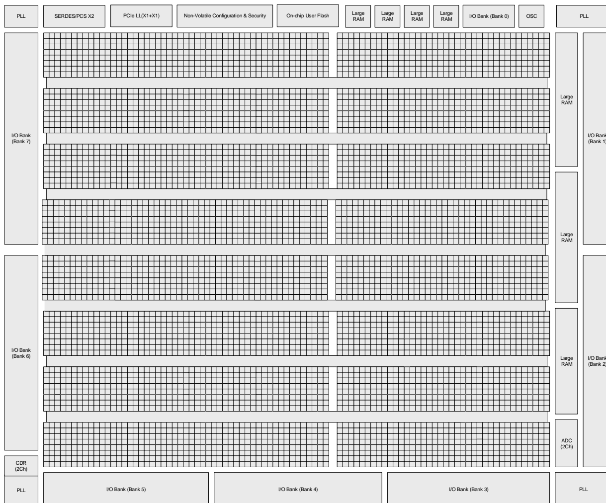
Figure 2.2. Simplified Block Diagram, MachXO5-NX-55T Device (Top Level)
