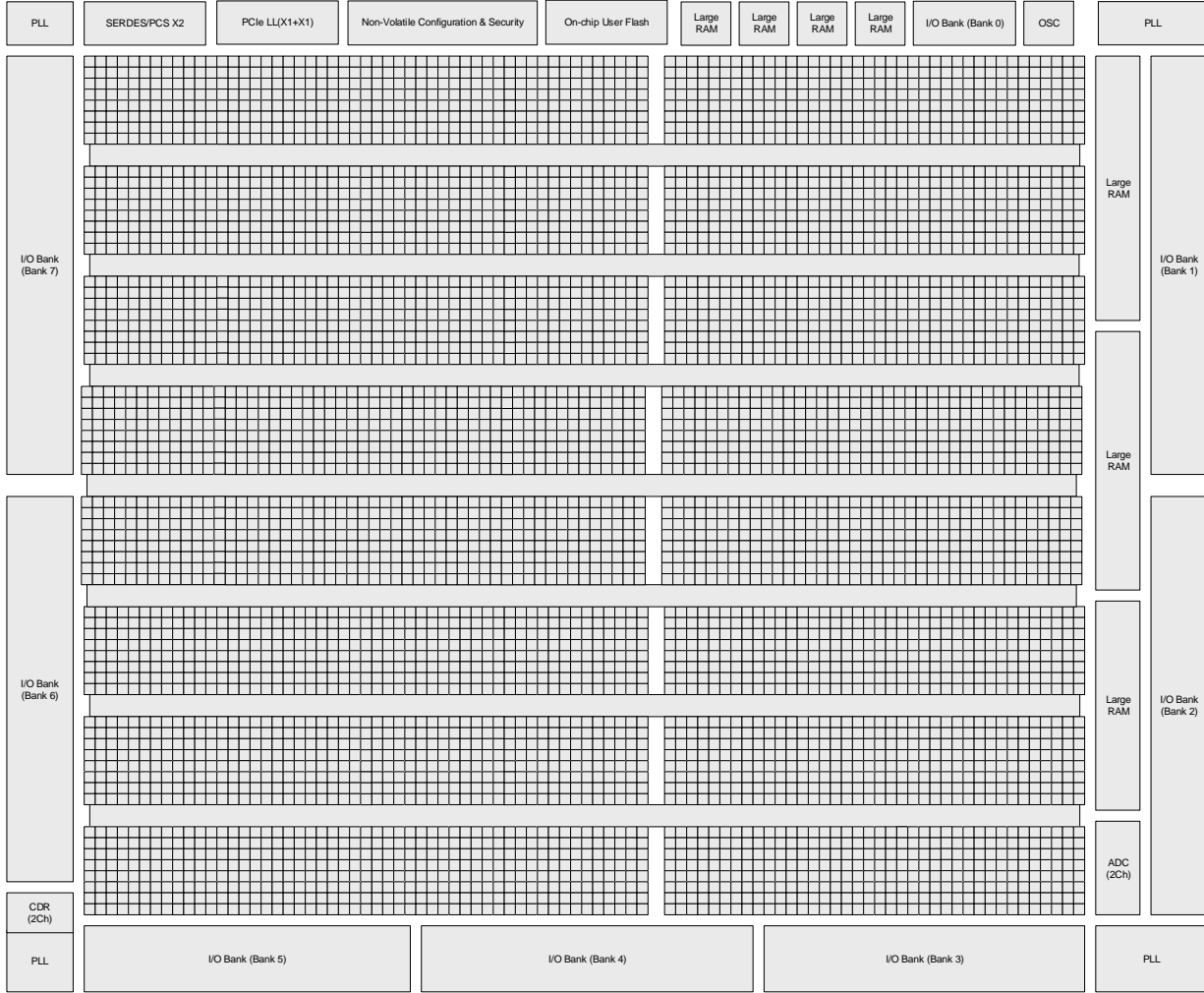
Figure 2.3. Simplified Block Diagram, MachXO5-NX-100T Device (Top Level)
