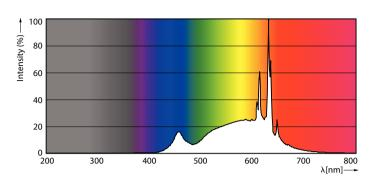
Spectral Power Distribution Colour - MASLEDspot VLE D 6.2-80W GU10 930 36D UK
