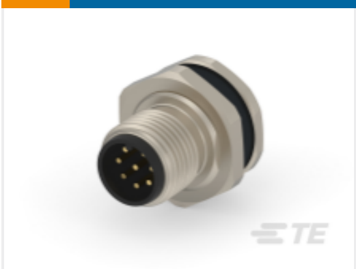
TE Part #T4171020008-001 M12,REAR MOUNT,MALE, A, 8P, 0.2M WIRE
