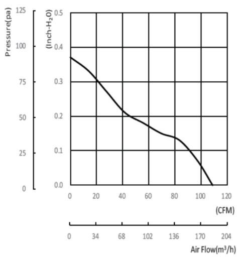
Air Flow & Static Pressure Curve
