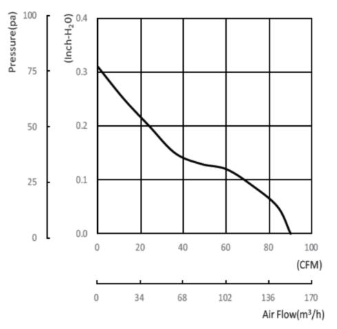
**Air Flow & Static Pressure Curve**
