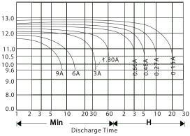
Note:Discharge shall be cut-off at 10.5V if discharge at 1CA and at 9.6V if at  ${\geq}1CA$
