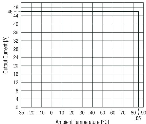
The module can be used in enclosed applications with full load, as long as the cooling is sufficient to keep the baseplate temperature at  $T_{CASE}$  below  $70^{\circ}C$ . The surrounding temperature should not exceed  $85^{\circ}C$ .
