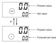
\* Each time the UP1 + UP3 or DW1 + DW3 are pressed, the sub-display will switch between the set value ("SET" is lit) and the forecast set value ("1" is lit).
