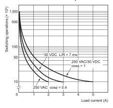
$\frac{\text{A maximum current of 0.15 A can be switched at 125 VDC (cos\phi = 1)}}{\text{and a maximum current of 0.1 A can be switched if L/R is 7 ms.}}$  In both cases, a life of 100,000 operations can be expected.
