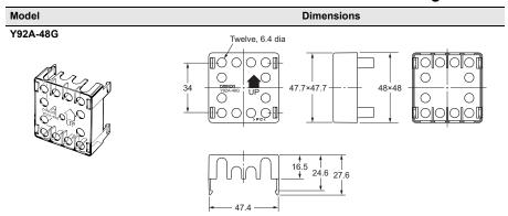
Note: The Terminal Cover can be used with a Back Connecting Socket (P3G-08 or P3GA-11) to enable finger protection.
