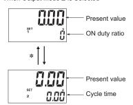
• Set each digit for the output time using the corresponding UP1 to UP3 Keys (DW1 to DW3 Keys). (The UP4 to UP6 Keys (DW4 to DW6 Keys) cannot be used.)
