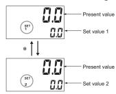
\* Each time the UP1 + UP3 or DW1 + DW3 are pressed, the sub-display will switch between set value 1 ("SET 1" is lit) and set value 2 ("SET 2" is lit).
