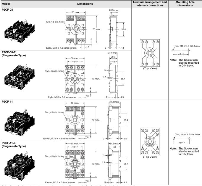
Note: Round crimp terminals cannot be used on Finger-safe Sockets. Use forked crimp terminals. The P2CF has hooks to fix the timer so the holding clips are not required.
