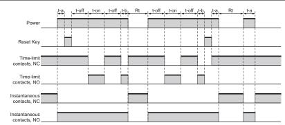
t-on = ON time, t-off = OFF time, Rt = Reset time (0.1 s min.),  $t-a \le t$ -off and  $t-b \le t$ -on (Indicates the time is less than the set time.)
