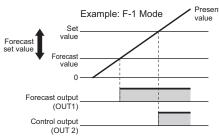
OUT1 (forecast output) turns ON when the present value reaches the forecast value.
