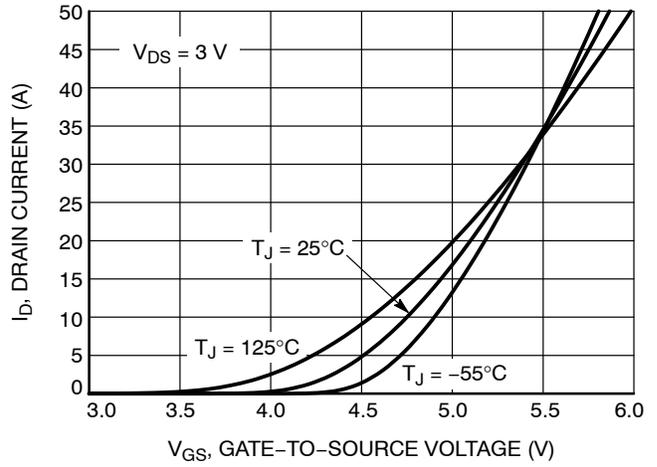
Figure 2. Transfer Characteristics
