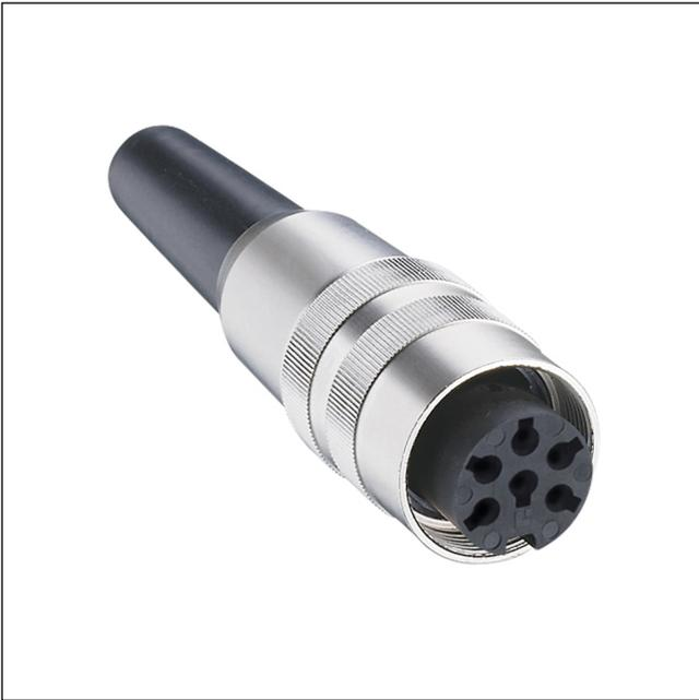
Socket acc. to IEC 61076-2-106, IP40, straight version, with threaded joint, empty housing for reception of crimp contacts, with bend protection, for cable diameter up to 6 mm
