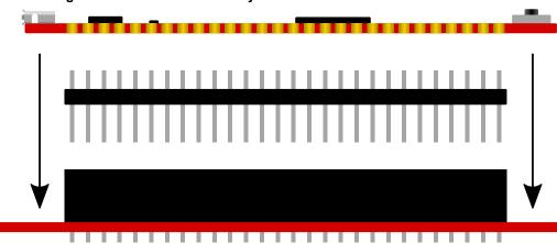
Figure 4-3. Connecting to Curiosity Nano Base for Click boards
