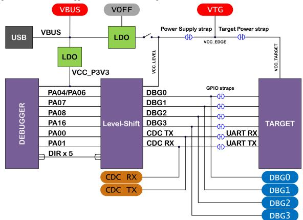
Figure 7-7. On-Board Debugger Connection Cut Straps
