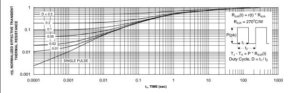
Figure 11. Transient Thermal Response Curve.
