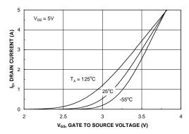
Figure 5. Transfer Characteristics.
