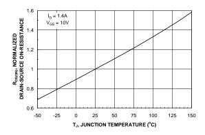
Figure 3. On-Resistance Variation with Temperature.
