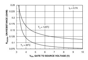
Figure 4. On-Resistance Variation with Gate-to-Source Voltage.
