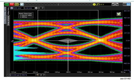
Fig. 11. HDMI 2.1 12G FRL eye diagram, WCM3; PCB without device; typical values
