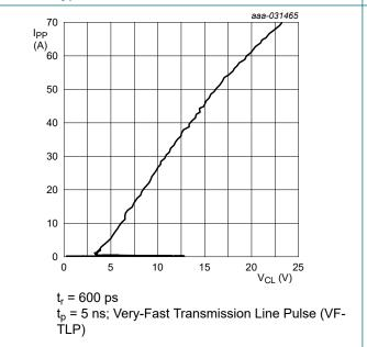
Fig. 14. Dynamic resistance with positive clamping; typical values
