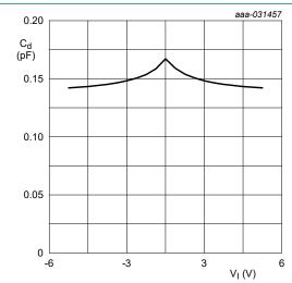
Fig. 6. Capacitance as a function of input voltage; typical values
