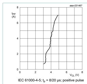
Fig. 16. Dynamic resistance with positive clamping; typical values
