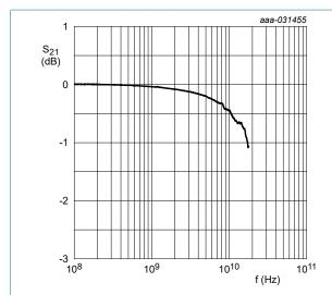
Fig. 4. Insertion loss; typical values
