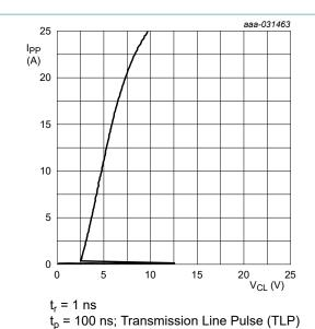
Fig. 12. Dynamic resistance with positive clamping; typical values
