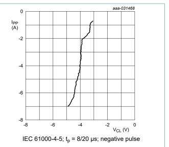
Fig. 17. Dynamic resistance with negative clamping; typical values
