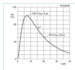
Fig. 2. 8/20 μs pulse waveform according to IEC 61000-4-5
