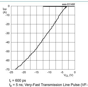
Fig. 15. Dynamic resistance with negative clamping; typical values
