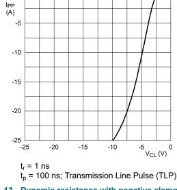
Fig. 13. Dynamic resistance with negative clamping; typical values
