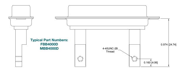
Power contacts can be offered with terminations suitable for use with bus bars.
