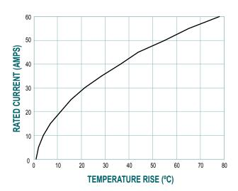
Test conducted in accordance with UL1977. All power contacts under load.
