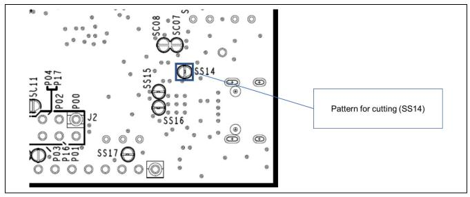
Figure 5-11 Position of the Pattern for Cutting (SS14)
