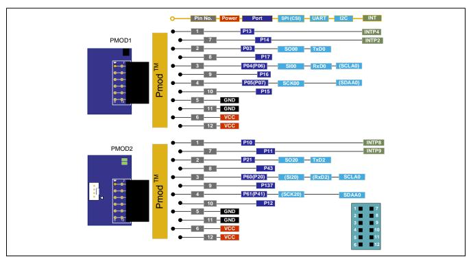
Figure 5-2, Table 5-3, and Table 5-4 show the pin assignments of the Pmod<sup>™</sup> connectors.
