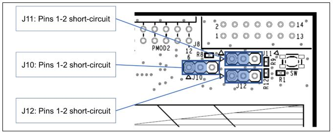
Figure 5-14 Settings for Use with COM Port Debugging (Top Side)
