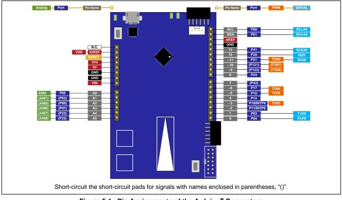
Figure 5-1 Pin Assignments of the Arduino<sup>®</sup> Connectors
