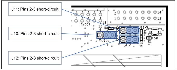
Figure 5-12 Settings for Use with the Emulator Connector (Top Side)
