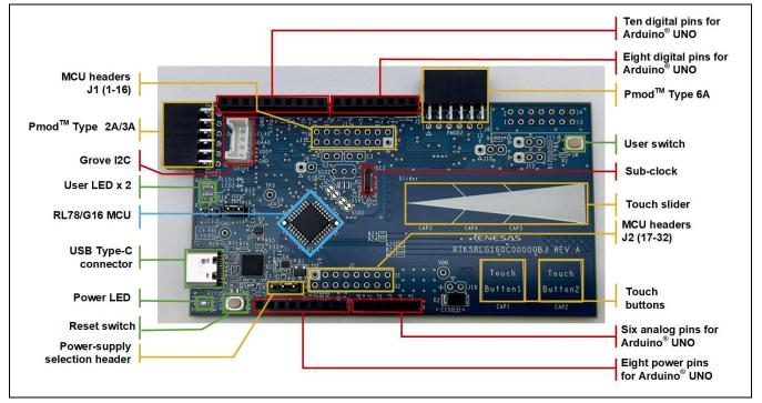
Figure 2-1 shows the external appearance of the top side of this product.
