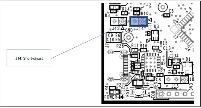
Figure 6-4 Settings for Use with COM Port Debugging (Top Side)
