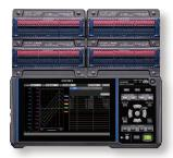
Configuration example: 120 channels of analog input
