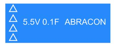
Example of the Markings of a 5.5V 0.1F supercapacitor
