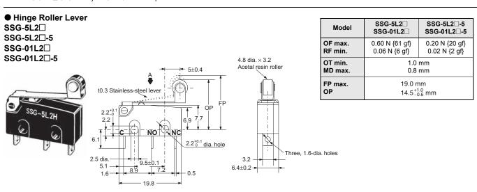
Note: 1. Unless otherwise specified, a tolerance of  $\pm 0.25$  mm applies to all dimensions.
