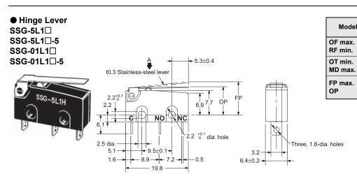
Note: Also available are models with a hinge lever length of 26.1 mm under the following model numbers; SSG-01L14□, SSG-5L14□, SSG-01L14□-5, and SSG-5L14□-5. Consult your OMRON sales representative for these models.
