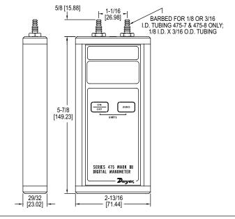
The Series 475 Intrinsically Safe Handheld Digital Manometer measures positive, negative, or differential pressures of air and natural gases in ranges from 1 in w.c. (0.249 kPa) to 150 psid (10.34 bar). The dual push pads on the front panel control the on/off, auto zero, and pressure unit selection, allowing for simple operation with no set up needed. When used with a Dwyer® Pitot tube (1), the Series 475 can also be used as an air velocity gage.
