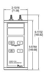
The Series 476A Single Pressure Digital Manometer can be used to measure low pressures from -20 to 20 in w.c. with ±1.5% full-scale accuracy.
