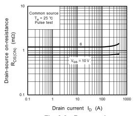
Fig. 8.8  $R_{DS(ON)}$  -  $I_D$
