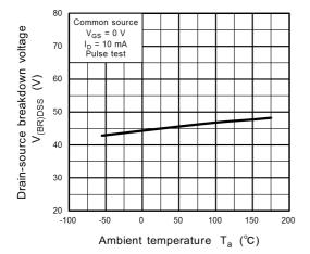
Fig. 8.11 V<sub>(BR)DSS</sub> - T<sub>a</sub>
