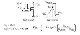
Fig. 8.16 Test Circuit/Waveform
