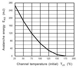
Fig. 8.15 E<sub>AS</sub> - T<sub>ch</sub>(Guaranteed Maximum)
