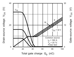
Fig. 8.14 Dynamic Input/Output Characteristics
