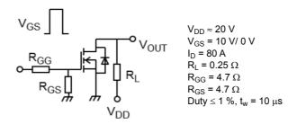
Fig. 6.2.1 Switching Time Test Circuit
