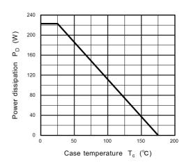
Fig. 8.19 P<sub>D</sub> - T<sub>c</sub> (Guaranteed Maximum)
