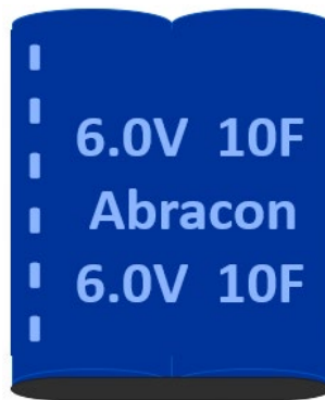
Example of the Markings of a 6.0V 10F supercapacitor
