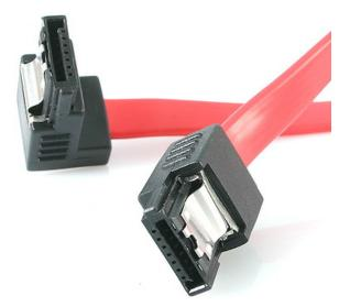
This 12in right-angled latching SATA cable features a (straight) female Serial ATA connector as well as a right-angled (female) SATA connector, providing a simple connection to a Serial ATA drive even if space near the drive's SATA port is limited. The cable offers latching connectors, which ensure secure connections for SATA hard drives and motherboards that support this feature.
