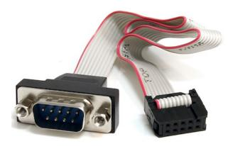
The PNL9M16 16-inch IDC Serial to Panel Mount Serial Cable, features a 10-pin (IDC) motherboard header connection on one end and a panel mount DB9 male connector port on the other - a simple answer for adding a DB9 (RS232) serial port to any computer system which has an RS232 serial panel mount receptacle.
