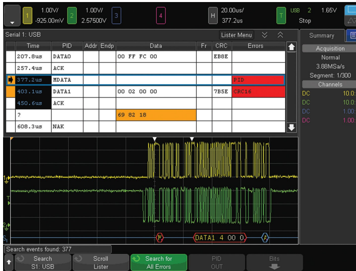
Figure 21. USB 2.0 trigger, decode and "lister" display.
