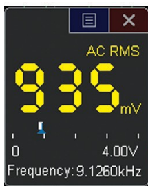
Figure 25. DVM 3-digit voltage and 5-digit frequency measurements always at your fingertips.
