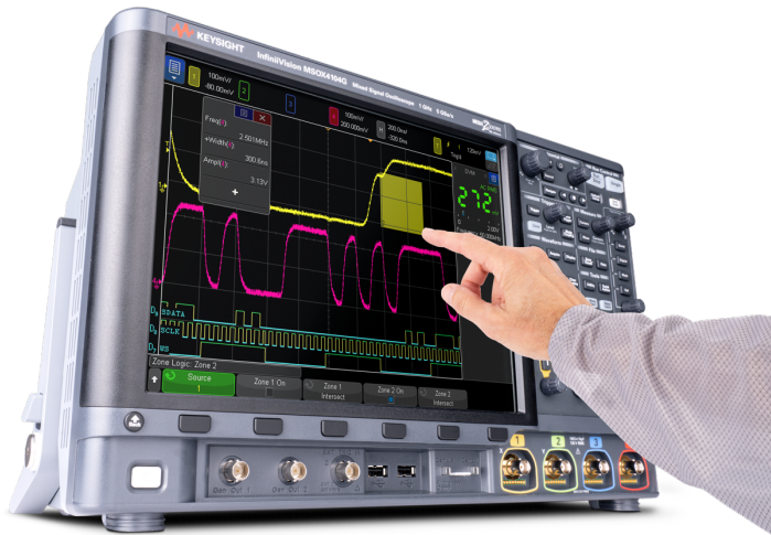
Figure 12. The 12.1-inch display and capacitive touch screen technology with large, touchable targets.
